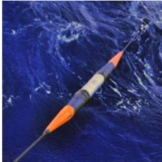
SMART cable sensor
